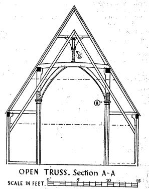
Fig. 21.—Section of open truss at Edgar's Farm, Stowmarket.
