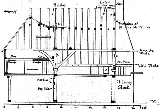
Fig. 18.—Lengthwise section of north end of building.
