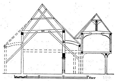
Fig. 20.—Section of open truss at Fyfield Hall, Essex.
